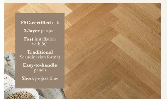
A high-quality floor that consists of three layers, with the wood fibres in each layer running in perpendicular directions to each other. This reduces the natural movement of the wood, providing a stable floor. Floor-locking technology, developed by sister company Välinge Innovation, ensures an easy and quick installation.
