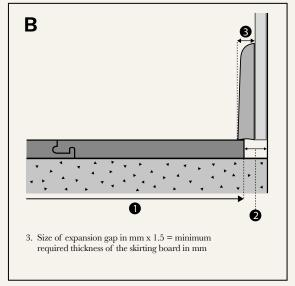
Make sure the floor can move freely under the walling panels.
