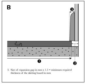
Make sure the floor can move freely under the walling panels.
